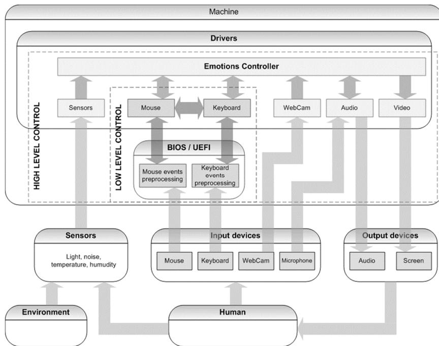
**Fig. 2.** Integration of the human-interface features on a personal computer architecture
