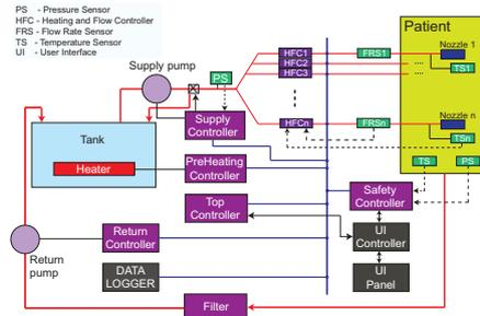
**Fig. 3.** The essential blocks of the proposed HIPEC equipment architecture
