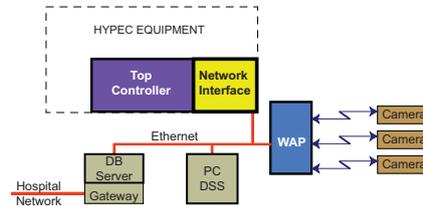
**Fig. 2.** The integrated HIPEC System
