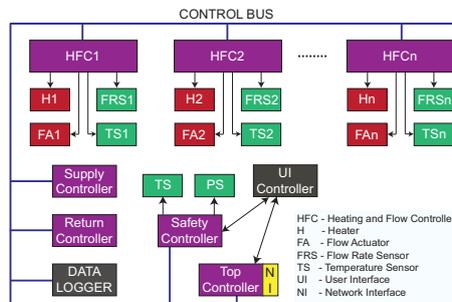
**Fig. 4.** Cyber part of HIPEC equipment as Cyber-Physical System
