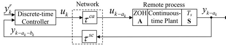
**Fig. 1.** Control system with network-induced time delay.
