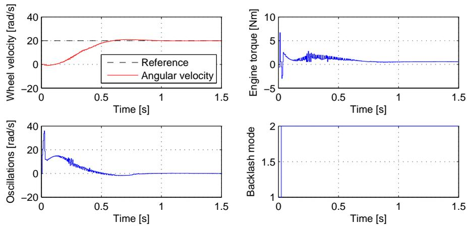
**Fig. 3.** a) Wheel angular velocity; b) Engine torque (control signal); c) Speed difference; d) Backlash mode.
