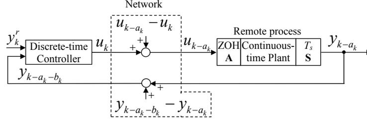
Fig. 2. Control system with network-induced time delay as disturbance.
